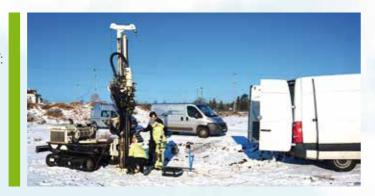
These technologies enable the collection of relevant in-situ-data for geological and hydraulic site characteristics as well as contaminant profiles during drilling operations. Using direct sense technology the strategy for the investigation of contaminated sites may be adapted dynamically during drilling campaign. This dynamic procedure leads to a considerable reduction of investigation time and investigation costs compared to conventional investigation strategies.
